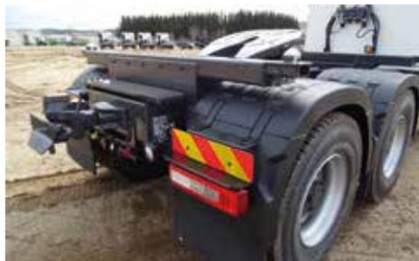
TRAVERSE ARRIÈRE CROCHET FORT TONNAGE - PLAQUE D'APPUI COL DE CYGNE
